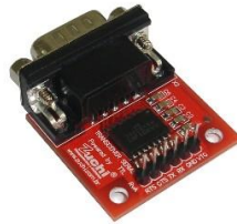
Transceiver Serial RS-232 EIA TTL 5V/3V3
