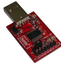
Conversor USB p/ Serial TTL 5V
